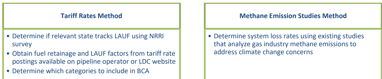
Figure 26. Methods for calculating gas system losses
